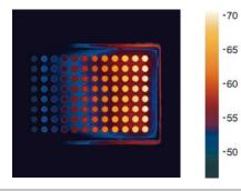
**Universal block for 0.2 and 0.5 ml tubes** Plate design delivers optimal heat transfer for both 0.2 ml and 0.5 ml tubes.
