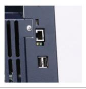
Ethernet port for LAN networking enables central protocol management across the network – always the correct protocol on each cycler.
